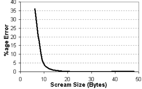
Figure 4. Percentage Error in SCREAM detection vs SCREAM size (bytes).
